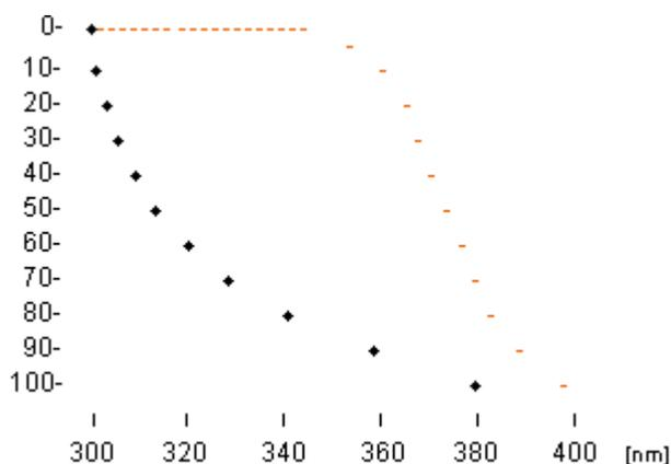
UV-Transmission of an alkyd varnish 100 µm wet film.
