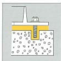
Machine Base Grouting
